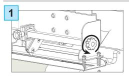
Remove the iron bar by unscrewing the black thumb screw.
