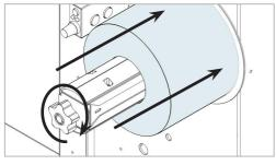
Load the lamination roll, move it along the supply shaft and make it match with the web, tighten the core holder.
