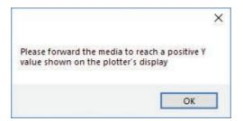
**Cause:** The starting Y position of the cut is a negative value (you can see coordinates on plotter's display when you move the media with arrows).
