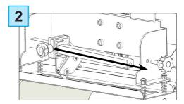
Slide the blade holder on or off. Replace the slide iron bar and rescrew the thumb screw.
