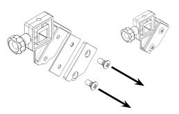
Remove the two screws holding the blade in place.
