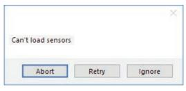
Cause: Media/Lamination sensors might be not plugged in correctly or turned off.
