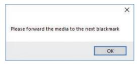
Cause: The starting Y position of the cut is a negative value (you can see coordinates on plotter's display when you move the media with arrows). Keep in mind also the offset influences the starting position of the cut. So, if you start the cut at Y coordinates 0, while you have an offset Y value of -10, you will still get this error. This error might happens when the media has been just loaded.
