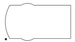
The cutting shape must be 100% black (otherwise in case of dashed lines, it must be a 100% magenta normal line) and have a thickness of 1 pt.
