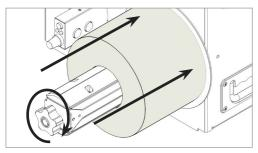
Load the printed roll against the disk. Tighten the core holder.
