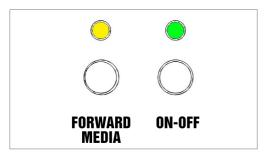
When both LEDs are off, the manual media feeding is active. It operates keeping pushed "Forward Media" button
