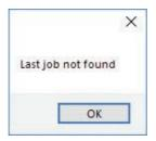
**Cause:** You will get this error when you try to open the last job when you run Cutting Manager for the first time after the installation.
