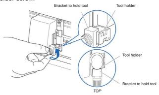
2. While pushing up the tool holder, push until its flange completely touches the upper part of the holder.
