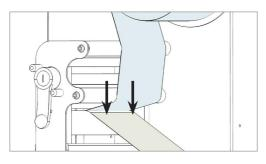
Hold the laminating film with both hands, pull it underneath the guide roller, center it and adhere the laminating film to the web.
