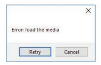
Cause: You launched the Cutting Manager while the plotter's lever was down.
