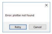
Cause: The plotter might be switched off or not properly connected.
