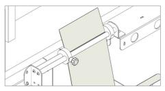
Pull the laminated media under the tension arm, then pass it between the aluminium rollers. The guide can be adjusted to prevent the media from shifting.
