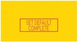
7. When the display shows "SET DEFAULT COMPLETE" turn off the plotter.
